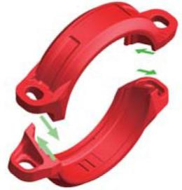
**T&G design:** The T&G (tongue & groove) mechanism provides a mechanical and frictional interlock resulting in a rigid joint which reduces undesired angular movement. ARGCO precision casting techniques allow the coupling segments to meet metal-to-metal when installed on properly grooved pipe.
