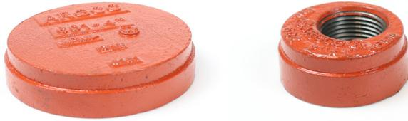
ARGCO Model 602 End Cap with Hole is an ideal transition fitting when a large reduction is required such as 6"×1", 4"×1" etc. The Model 602 can be used as an alternative to expensive swaged nipples.
