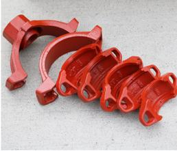
**Ductile Iron:** Standard coupling housings and fittings are made of ductile iron conforming to ASTM A536 Gr. 65-45-12. The properties of Grade 65-45-12 ductile iron are as follows; 65,000 psi (448 MPa) tensile strength, 45,000 psi (310 MPa) yield strength and 12% elongation. As an option we also offer ductile iron made to ASTM A395 Gr. 60-40-18, for applications where required or where boiler codes may apply.
