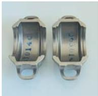
**Stainless Steel:** ARGCO offers a variety of stainless steel casting materials depending on your intended application. Standard coupling housing and fitting materials include CF8 (304), CF8M (316) or CF3M (316L) per ASTM A743. Optional materials include 2205 Duplex, 2507 Super Duplex and ASTM CK-3MCuN (UNSJ93245), equivalent to 254SMO\*. (\* 254SMO is a registered trademark of Avesta Polarit AQB.) Most of these materials are special order. Call your sales rep for details.
